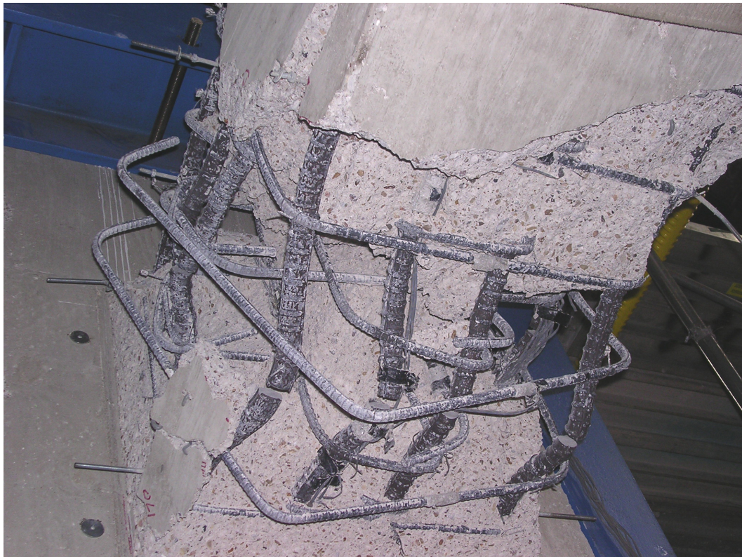
Figure 4.8 Opening of Hoops in Specimen S24-1UT
