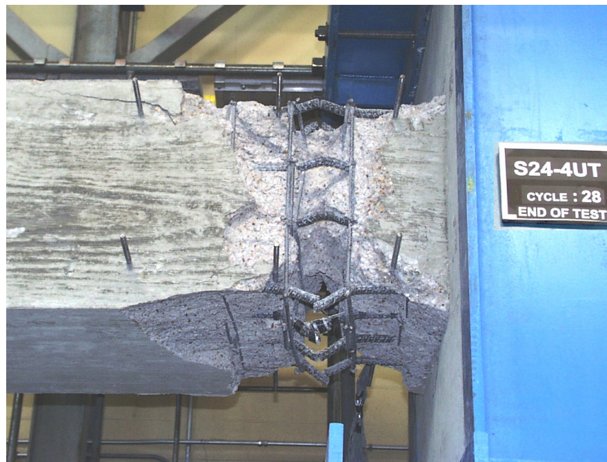
Figure 6.1 Longitudinal Bar Buckling in Specimen S24-4UT
